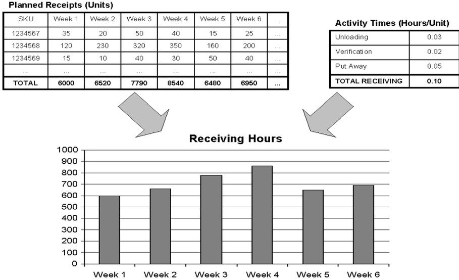
Figure 2.2: Conversion of planned receipts into receiving hours.
